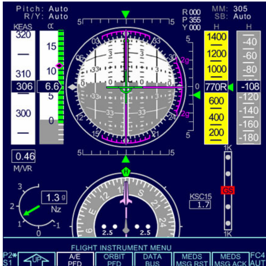
Figure 2.11-2 Typical A/E PFD during approach/land
