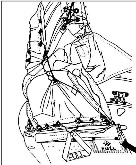
PACKED VALISE HANGING OFF SIDE HATCH PRIOR TO SLIDE DEPLOYMENT
