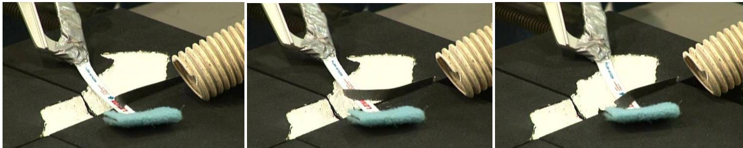
Figure 3 – After each cut along a damaged/undamaged site, remove hacksaw and reposition for the next cut
