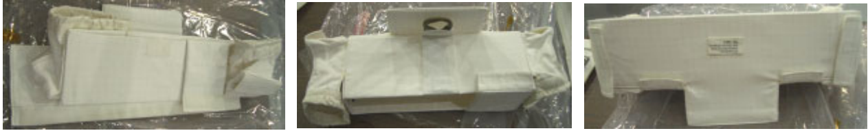
Figure 5 – Temperature sensor insert folded for launch and assembled
