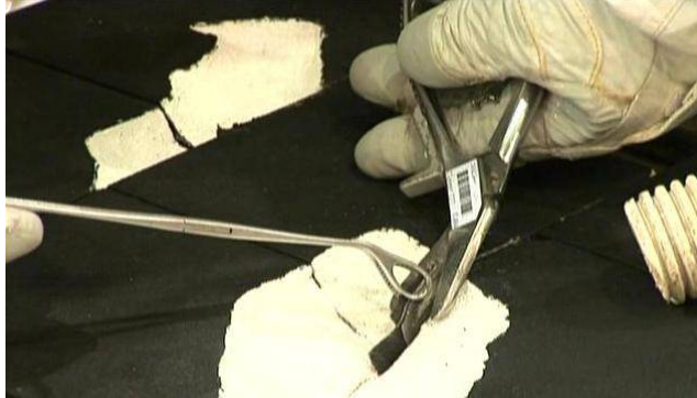
Figure 4 – Note, analysis may indicate that there is no need to remove gap filler from a damaged area prior to tile repairs
