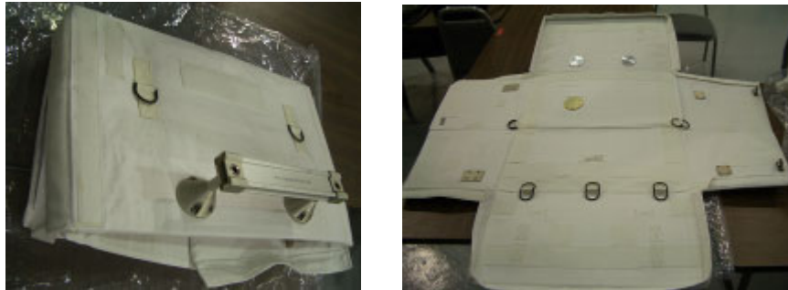
Figure 1 – RCC crack repair bag exterior, folded for launch, and unfolded for assembly
