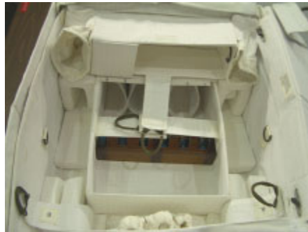
Figure 6 – Interior bag tool inserts installed
