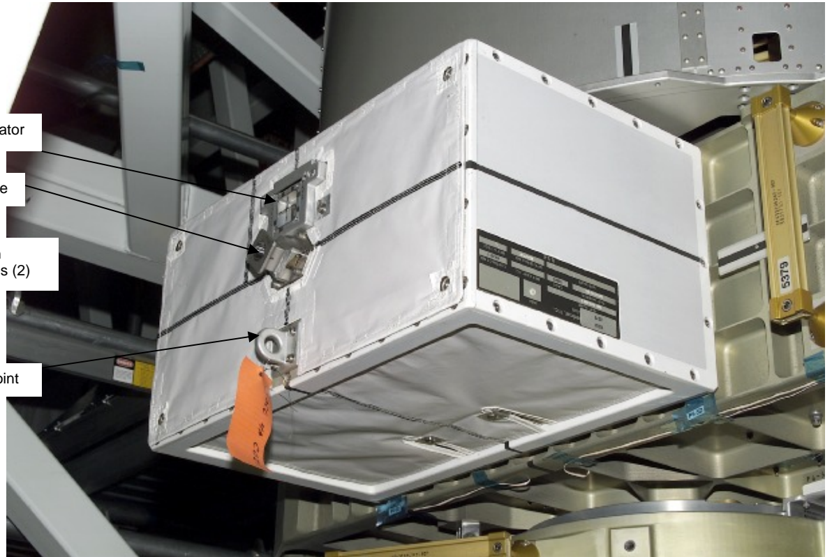
ECU Installed on Platform Assembly
