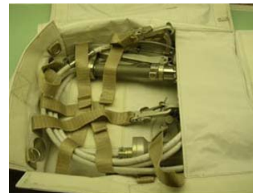
Vent tool & VTE Installed in VTE Bag
