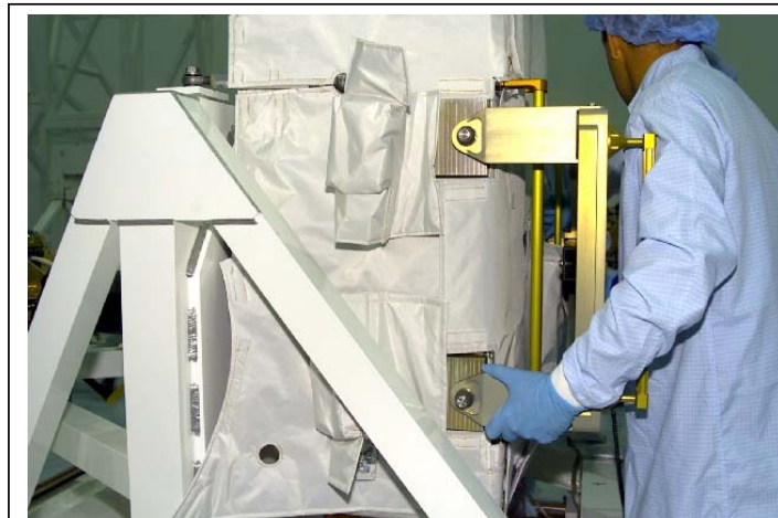
AGB INSTALL ON FHRC – DOUBLE PIN SIDE (MLI FLAPS ARE VELCROED OPEN)
