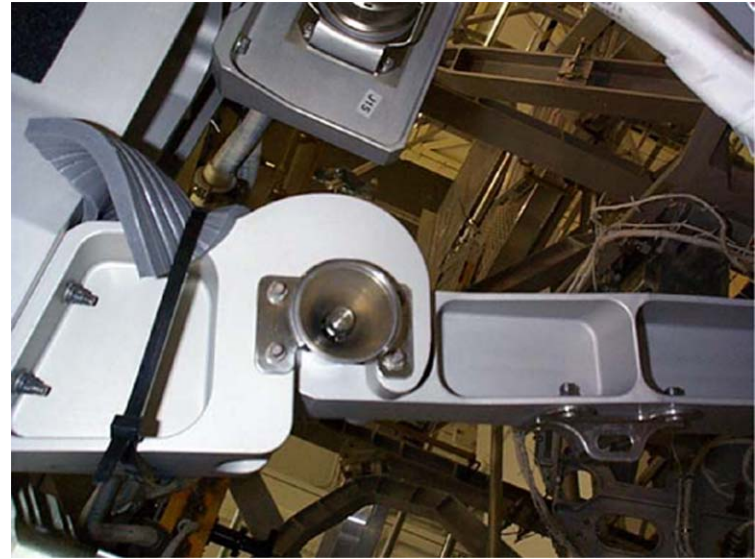
SARJ Brace Cup Cone placed in on-orbit position
