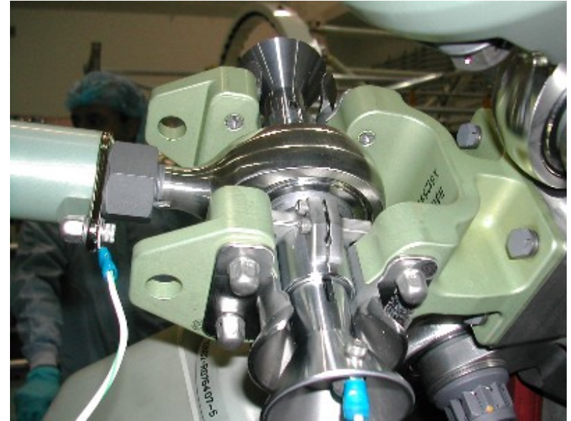
AJIS Strut Cone Fastener (engaged, but not fastened)
