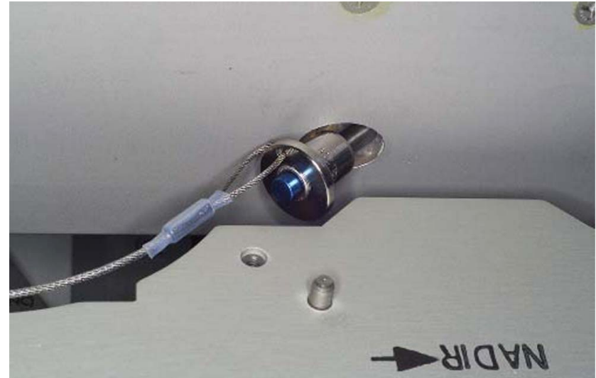
P1 MT Stop PIP Pin Fully Inserted (showing clearance to MT envelope)
