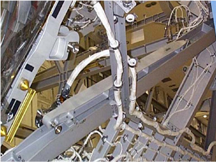
SARJ Brace (Launch position)
