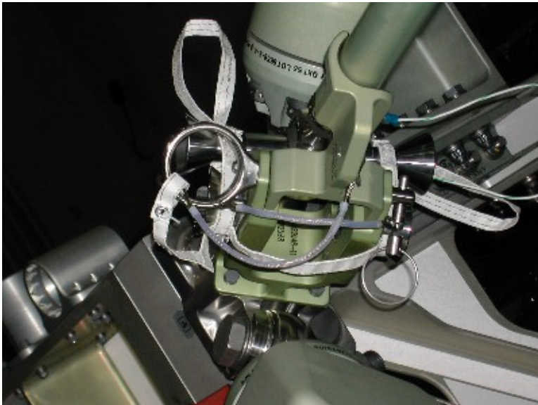
AJIS Strut with Strut Launch Restraint (thermal bootie removed)
