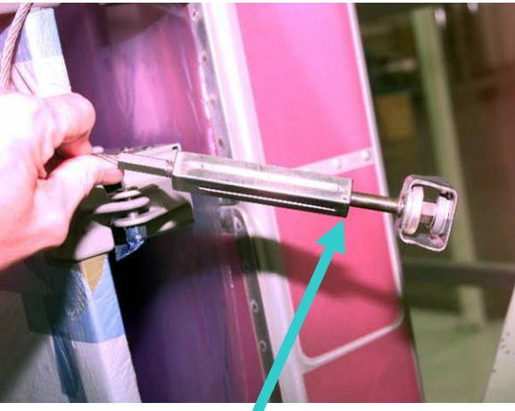
Figure 2. Uninstalled Cinch – bolt needs to catch last thread in square boss in order for cinch to retract properly. Pulling on bolt should show no movement
