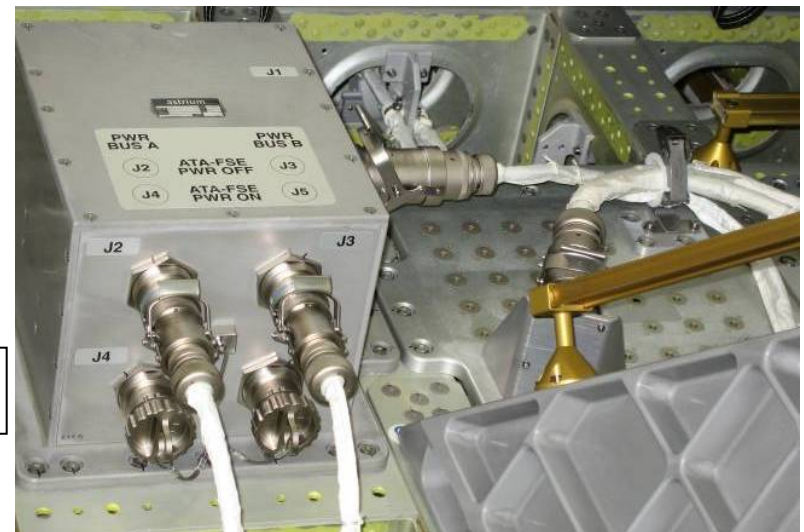
ESP-3 Shuttle Power Cable P1 to dummy receptacle of KYA – Landing Config
