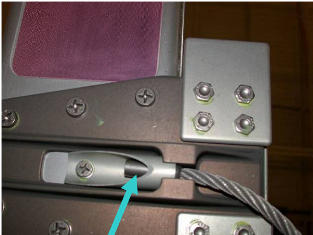
Figure 1. Fixed end of cinch cable fully seated in retention bracket
