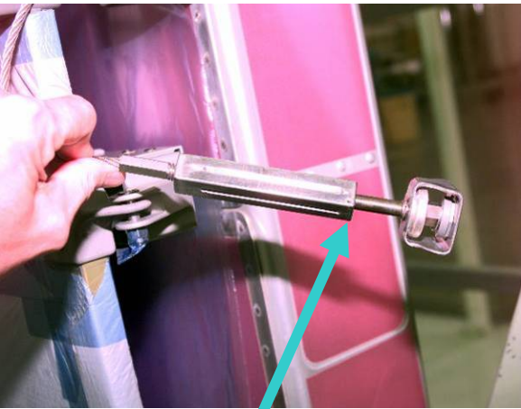
Figure 2. Uninstalled Cinch – bolt needs to catch last thread in square boss in order for cinch to retract properly. Pulling on bolt should show no movement
