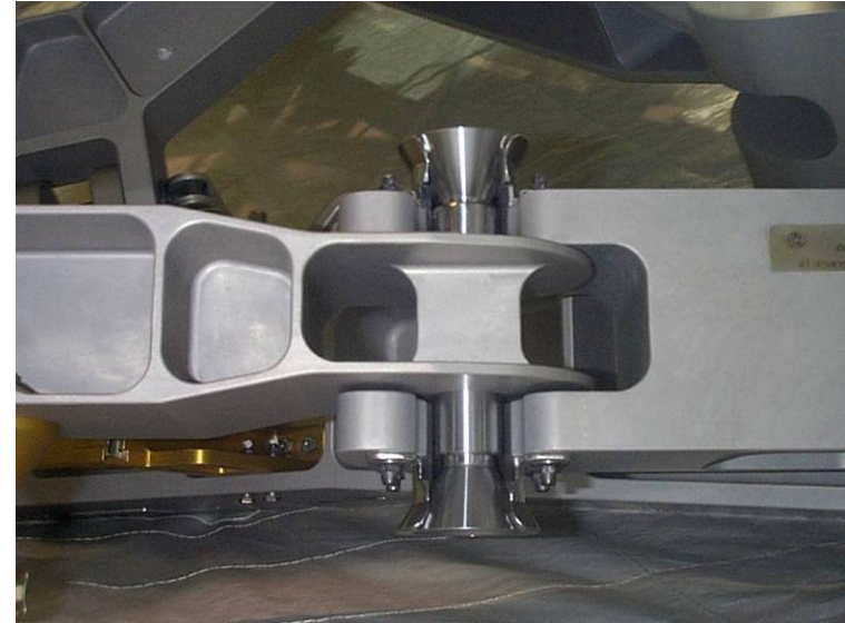
Figure 10. Diagonal and SARJ braces Jack-Joint cup-cones
