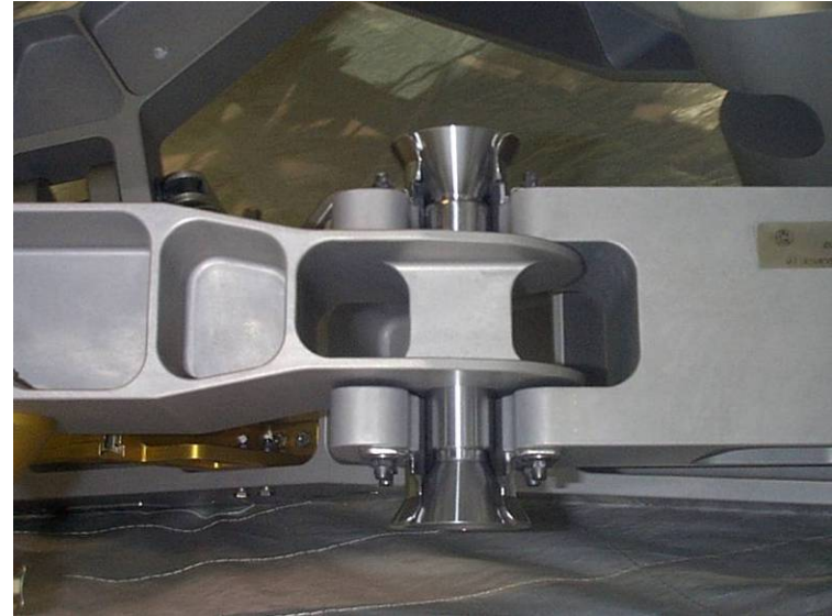
Figure 10. Diagonal and SARJ braces Jack-Joint cup-cones
