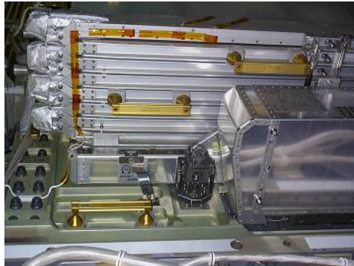
PV Radiator – MDA H32 Fastener Located Near Ground Strap
