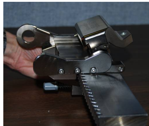
Figure 8. Mount Assy on Race Ring, mount leg clamp open (initial position)
