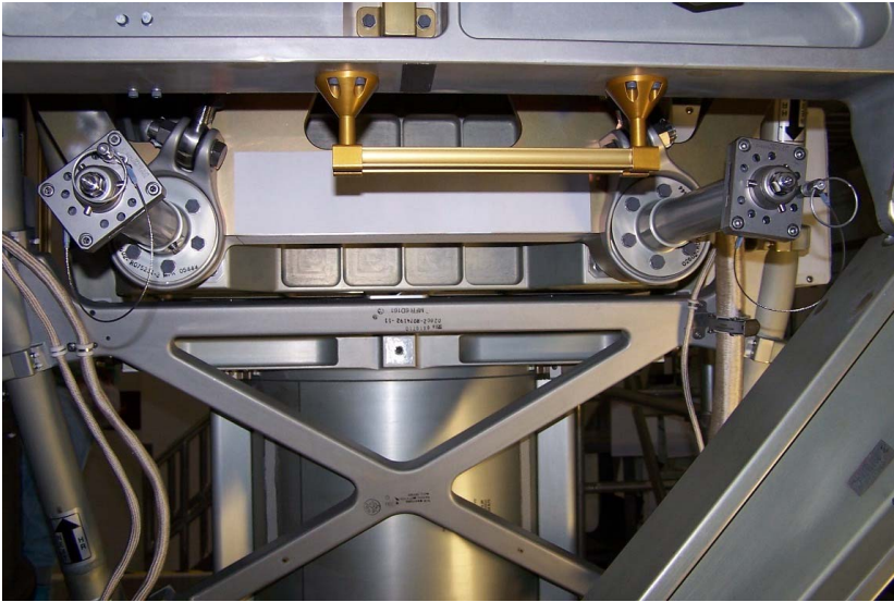
Aft Beta Gimbal Restraints and IEA Keel Structure
