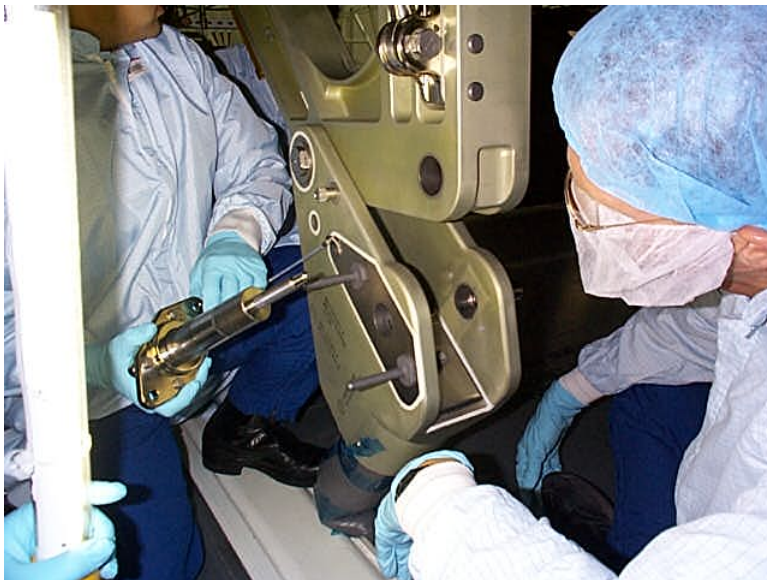
Aft Beta Gimbal Restraints and IEA Keel Structure
