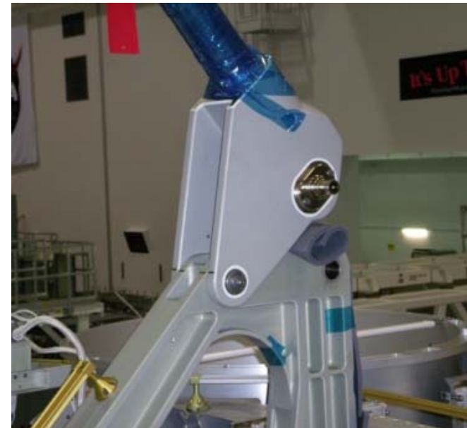
Beta Gimbal Restraints and IEA Keel Pin
