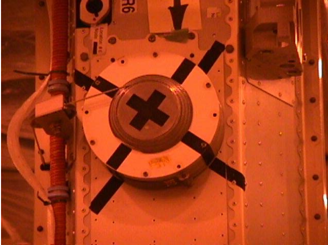
SABB Tensioning Reel Outboard – markings not on S6
