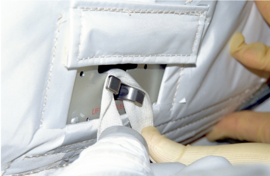
PETAL LAUNCH RESTRAINT RELEASE USING ADJUSTABLE TETHER STRAP
