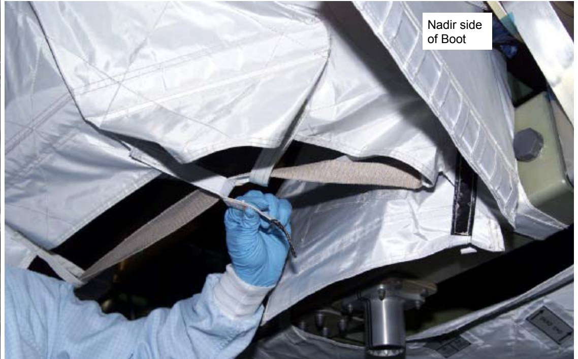
Final Step – black Velcro strap on nadir end of shroud routed through 2nd guide strap belt loop
