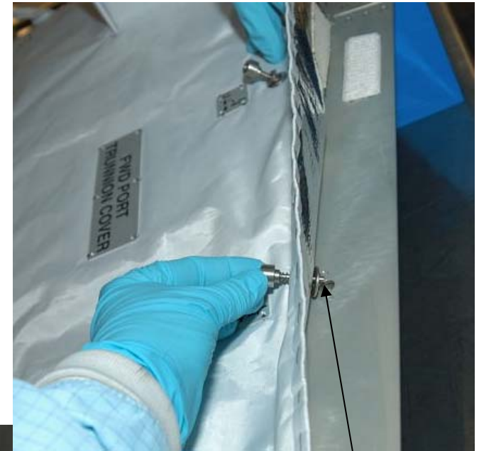
TRUNNION COVER – mounted to test fixture
