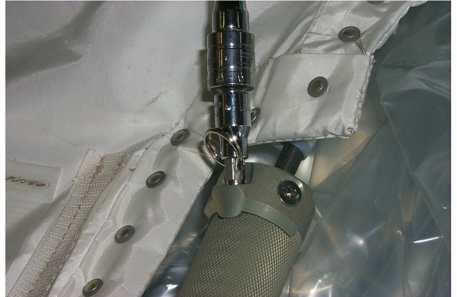
TOOL INTERFACE WITH TURNBUCKLE PIP PIN
