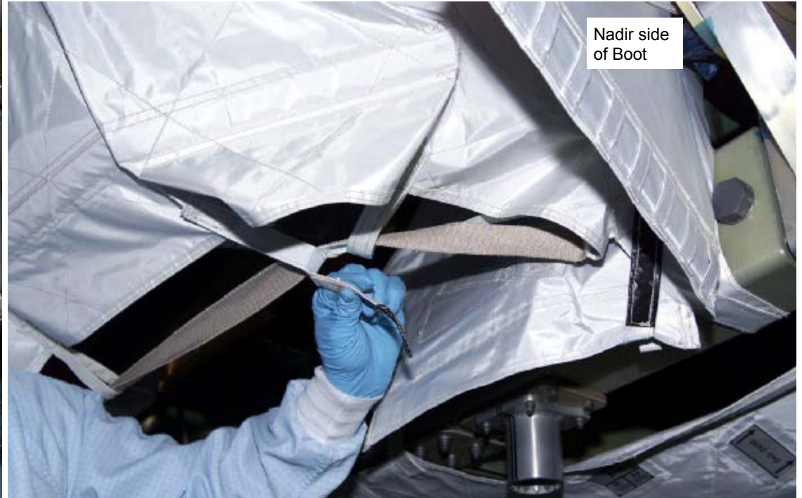
Final Step – black Velcro strap on nadir end of shroud routed through 2nd guide strap belt loop
