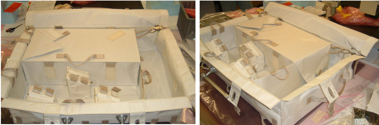
Figure 3.- Fully assembled Sample Bag with DTO insert
