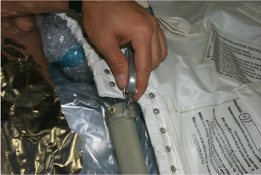
TETHER INTERFACE WITH TURNBUCKLE PIP PIN RING
