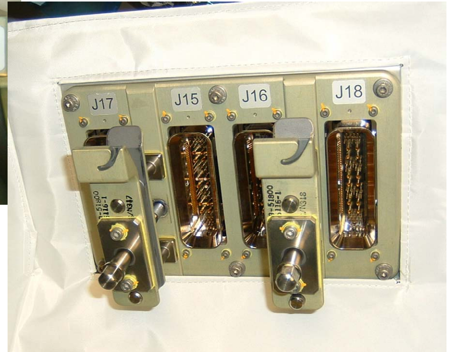
Horseshoe connectors released and removed
