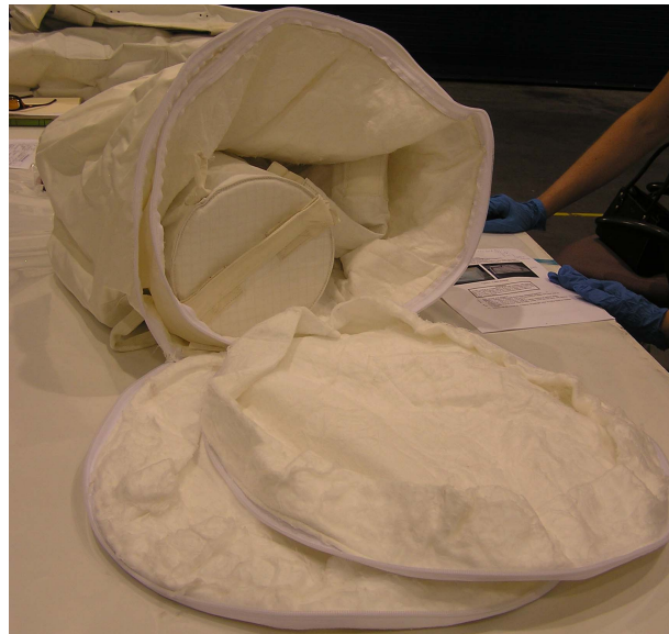
Figure 1.- T-RAD Stowage (Containment Bag on Left, Nomex Sacks (2) on Right)
