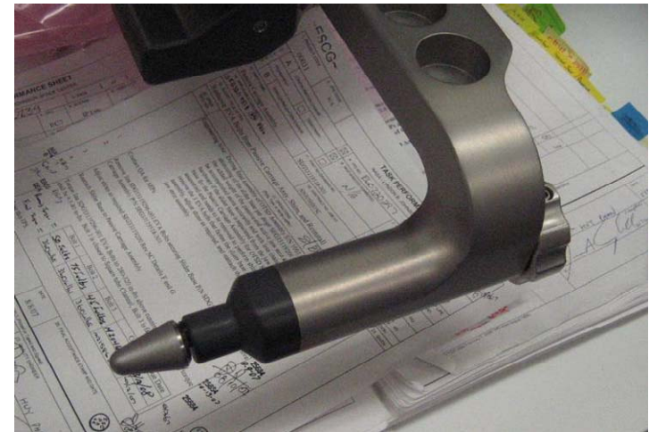
2-pin side in RELEASE position
