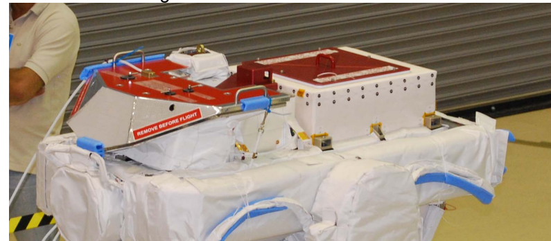
“Remove before flight” covers on SOLAR sensors
