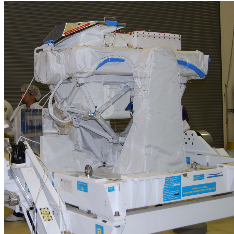
“Remove before flight” covers on SOLAR sensors
