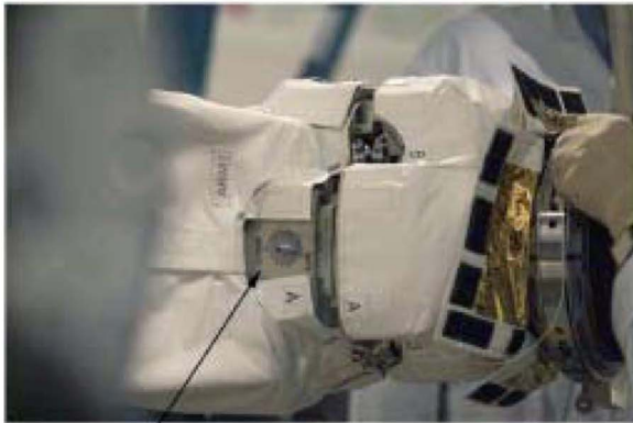
Connector Mate/Demate Visual Cue at Shoulder
