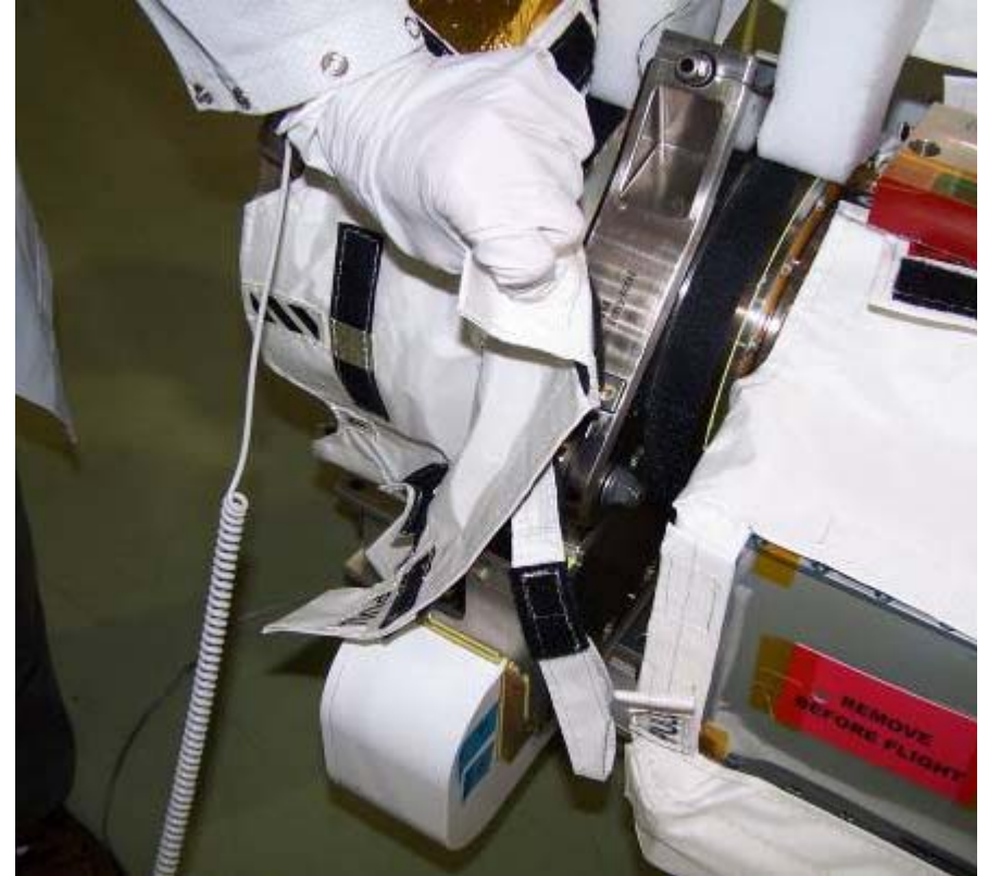
Wrist MLI (install barber poll and solid black line sides first)
