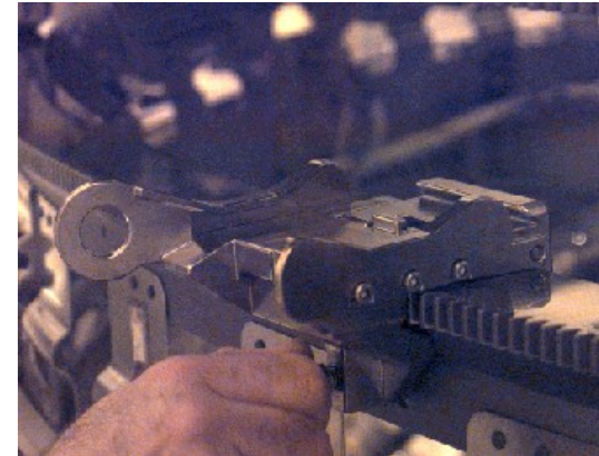
Mount Assy on Race Ring, mount clamp leg closed (final position)
