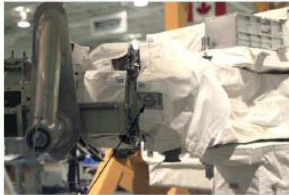
Connector Mate/Demate Visual Cue at Shoulder
