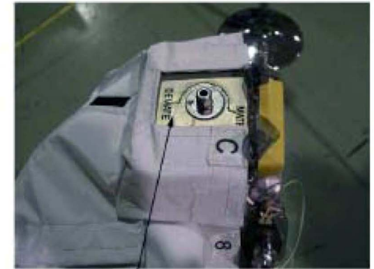
Connector Mate/Demate Visual Cue at Shoulder
