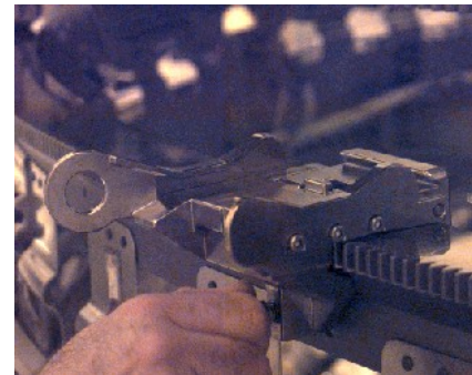
Mount assembly installed on SARJ ring
