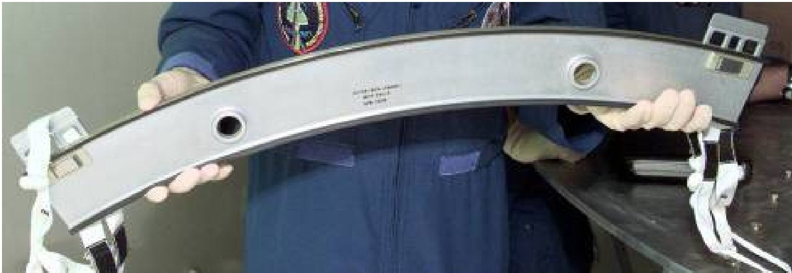
PCBM Contamination Cover
