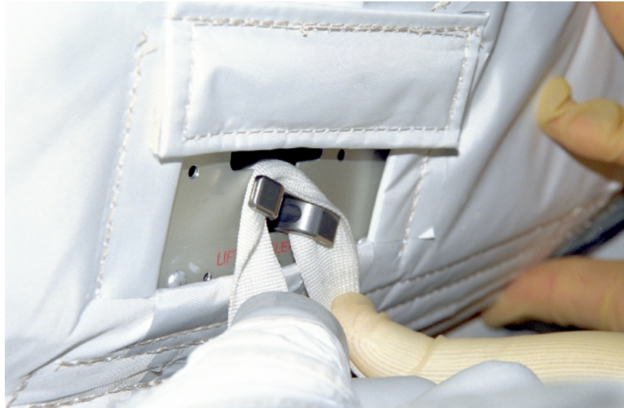
PETAL LAUNCH RESTRAINT RELEASE USING ADJUSTABLE TETHER STRAP
