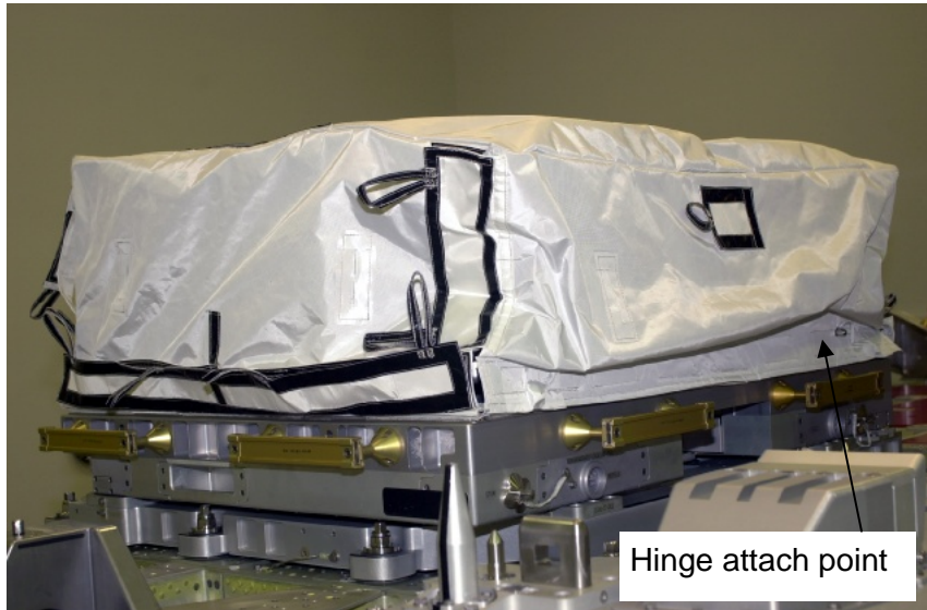
Spare MBSU w/MLI attached to FRAM on ESP2
