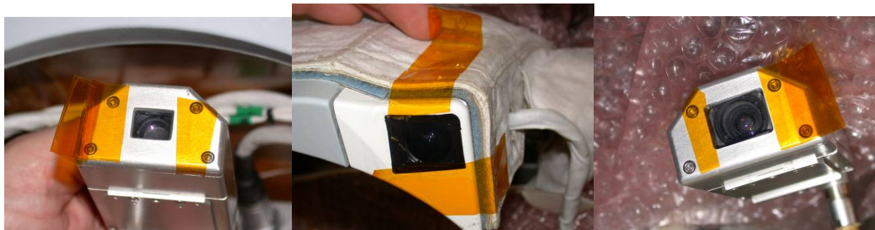
Figure 2 - ERCA lense covered with Teflon squares and Kapton tape
