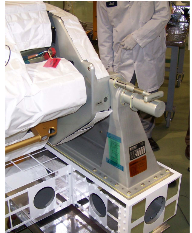
LEE Brace Retention Assembly (disengaged)
