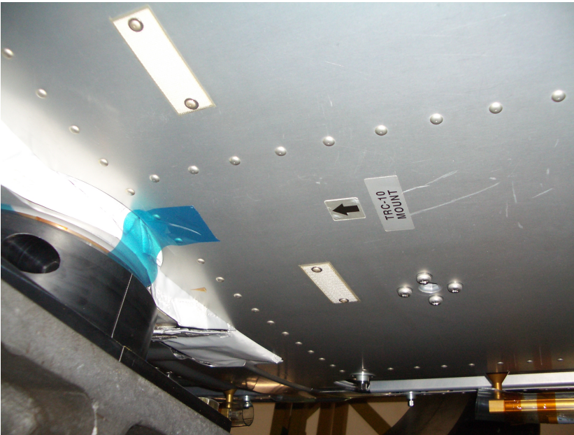
JLP keel (TRC-10) align arrow and Velcro
