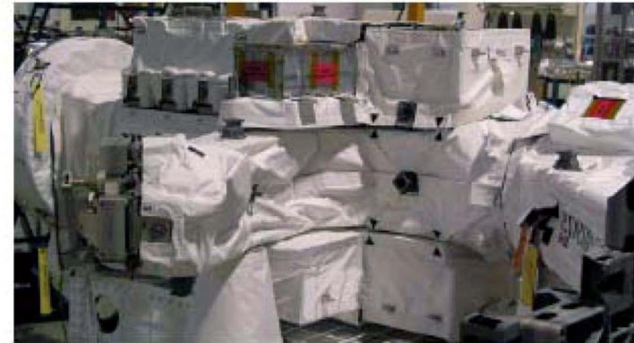
EP #1 and EP #2 assembled to Upper Body Structure
