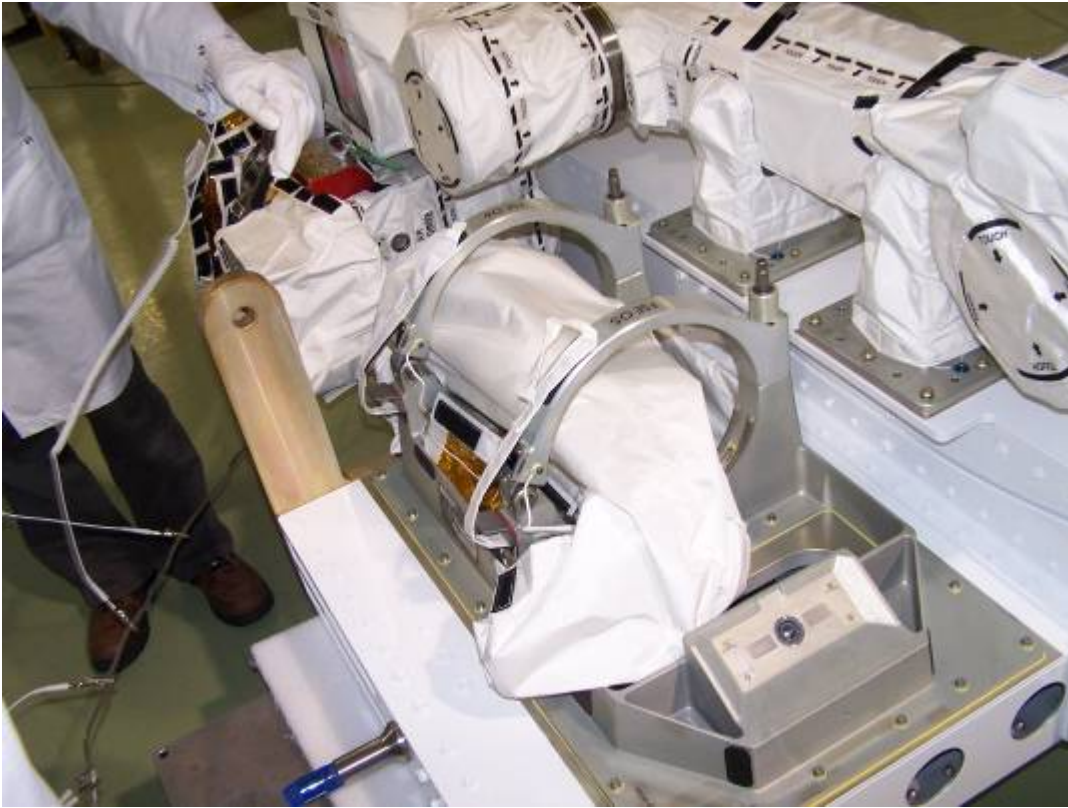
OTCM FSE landing configuration (before KA installed)
