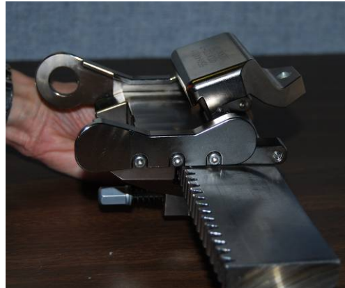
Mount Assy on Race Ring, mount clamp leg open (initial position)
