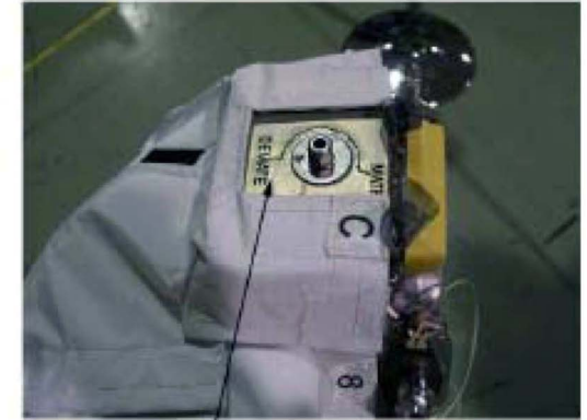
Connector Mate/Demate Visual Cue at Shoulder
