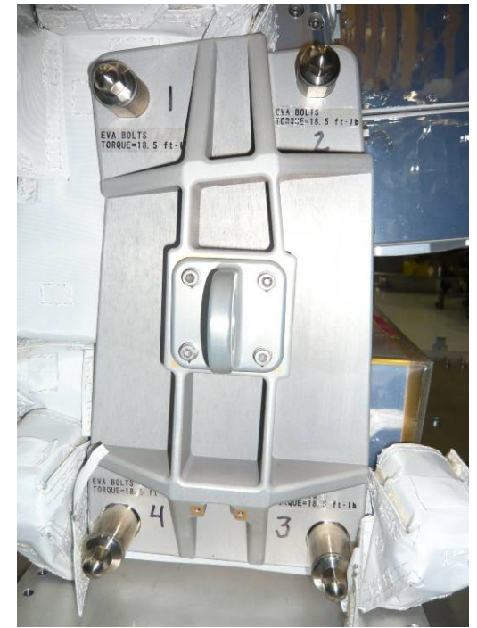
Launch Lock Installed (Labeling Shown)
