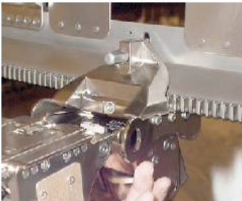
Slot in Race Ring to align Mount Boss
