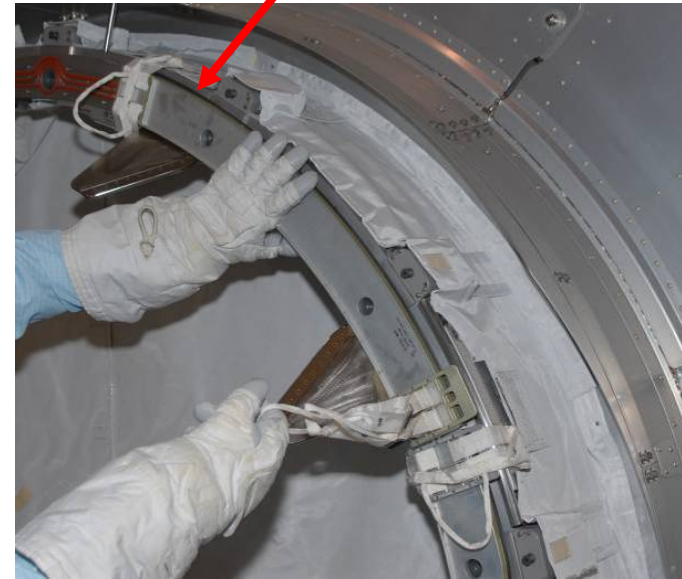
Contamination Cover Installed (8 in total)
