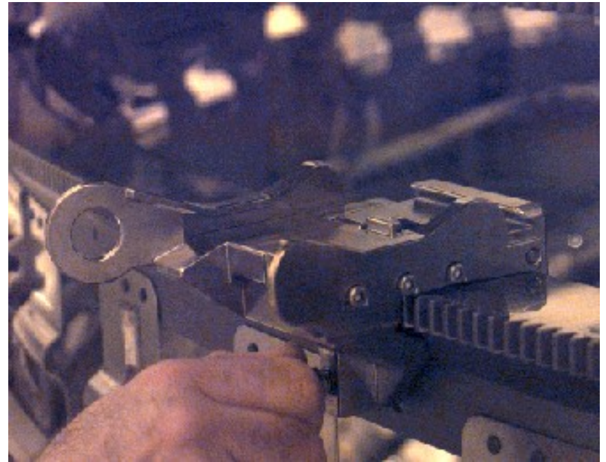
Mount assembly installed on SARJ ring
