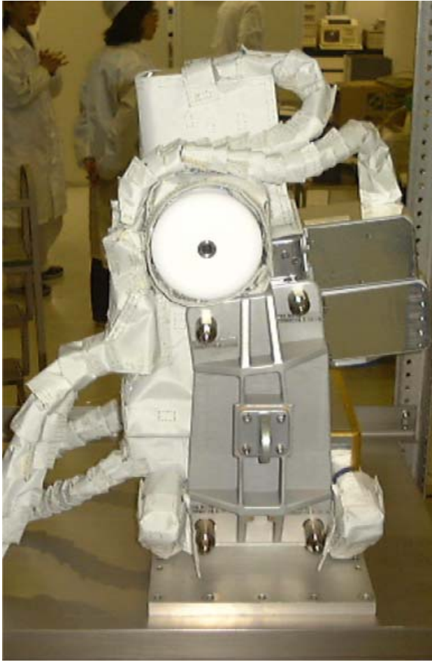
Launch Lock Installed
