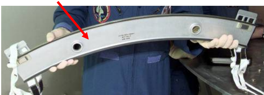
Contamination Cover Removed (8 in total)
