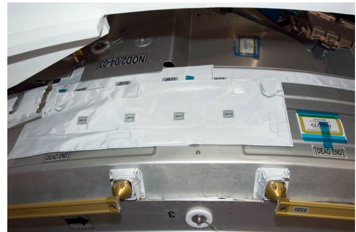
Node 2 MLI blanket section, pre-flight
