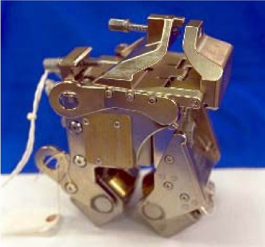
Trundle bearing and mount assembly
