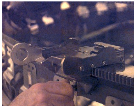
Mount assembly installed on SARJ ring
