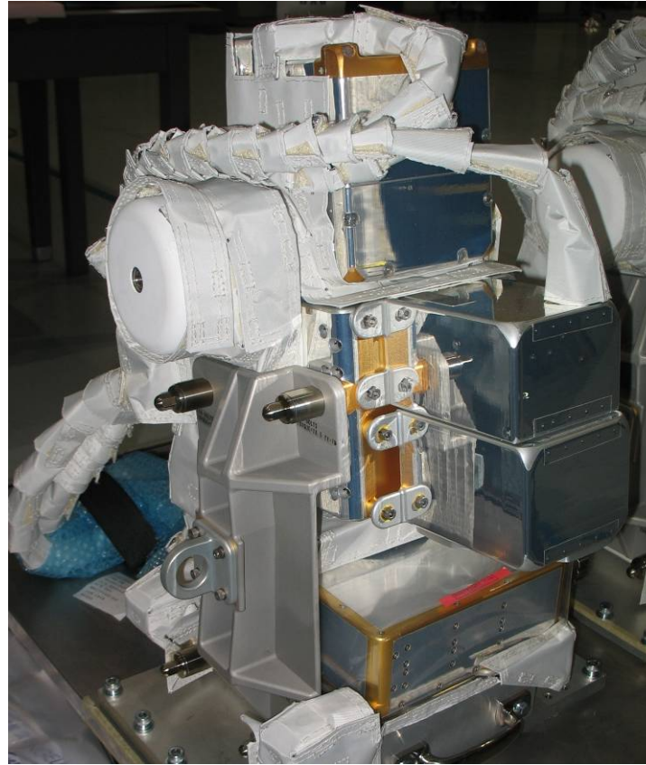
Launch Lock Installed (MLI Removed)
