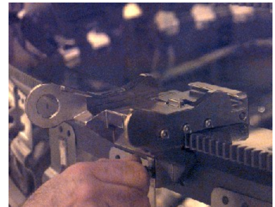
Mount Assy on Race Ring, mount clamp leg closed (final position)
