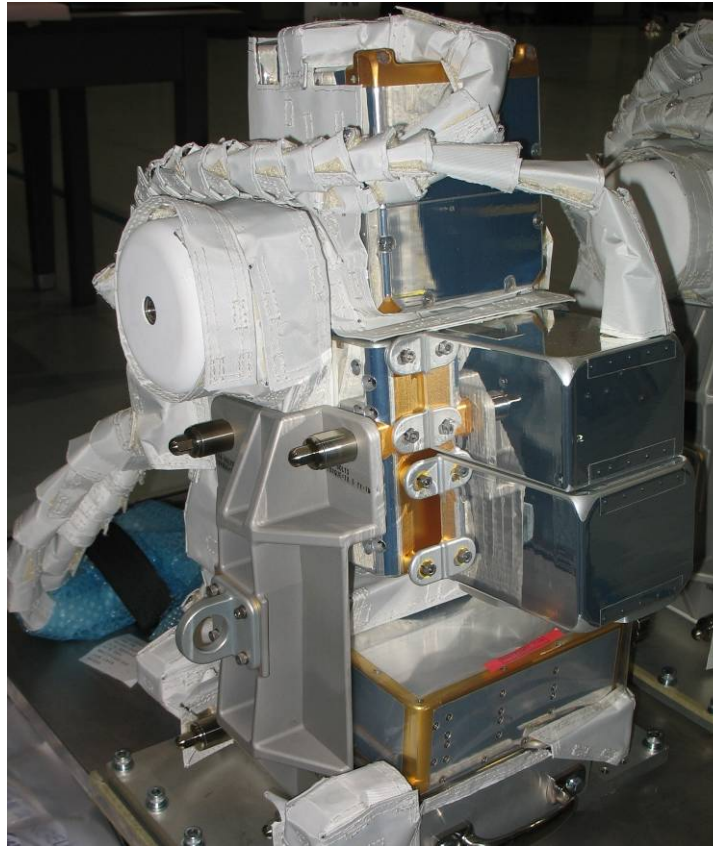
Launch Lock Installed (MLI Removed)
