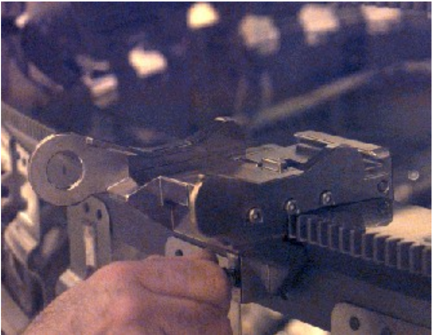
Mount assembly installed on SARJ ring
