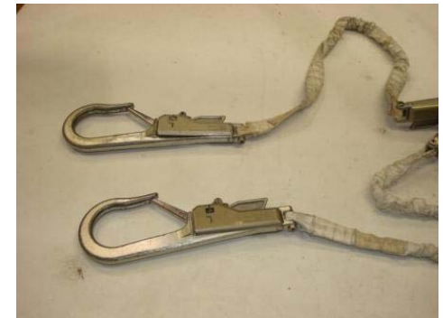
2 large waist tether hooks to port ODS handrail
