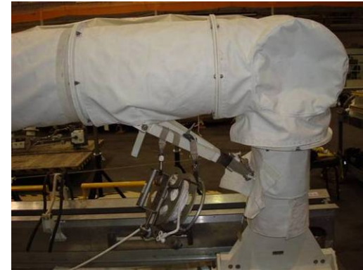
Rope Reel temp stowed on SRMS shoulder brace with AET at end of EVA1
