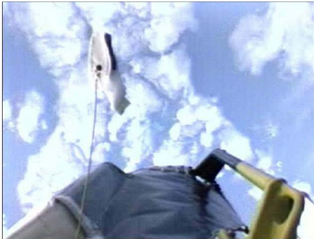
Figure 1. Grounding Tab Obstructing Camera View
