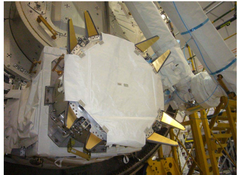
Figure 2. EFBM Center Disk Cover Installed
