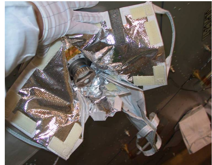
Figure 4. Close up of Connector MLI Open
