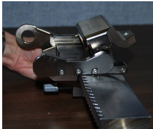
Figure 11. Mount Assy on Race Ring, mount leg clamp open (initial position)
