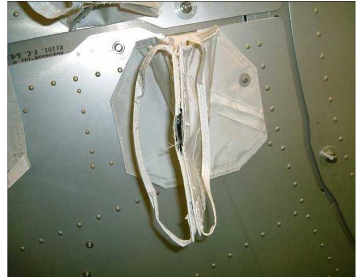
Figure 3. Close up of Connector MLI Closed
