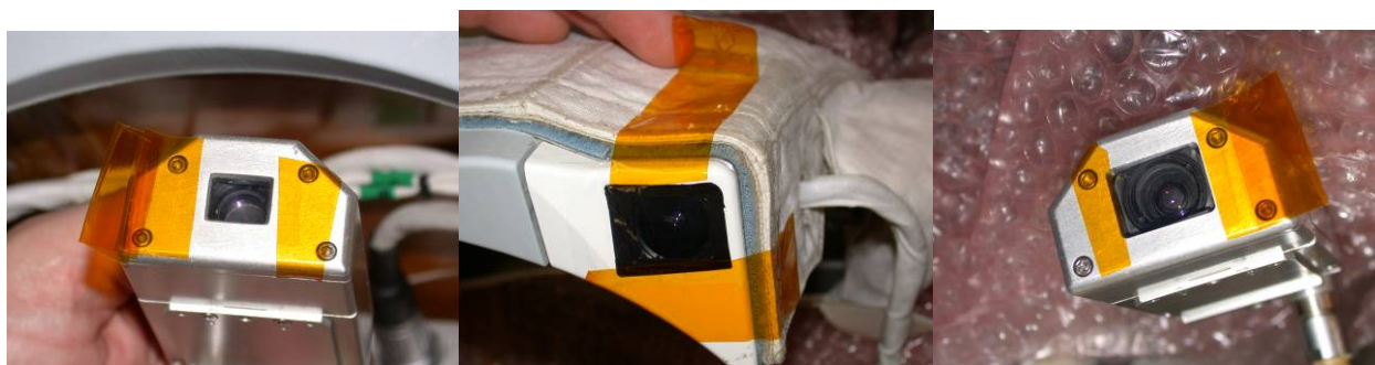
Figure 2 - ERCA lenses covered with Teflon squares and Kapton tape
