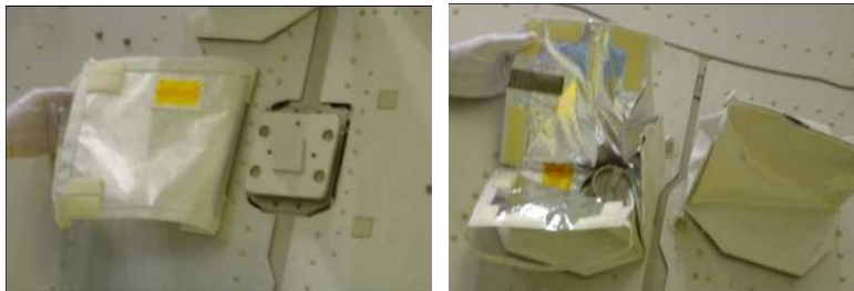
Figure 2. GPS Antenna MLI Covers Opened
