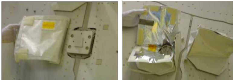
Figure 2. GPS Antenna MLI Covers Opened
