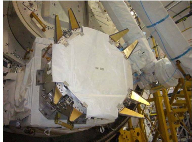
Figure 2. EFBM Center Disk Cover Installed
