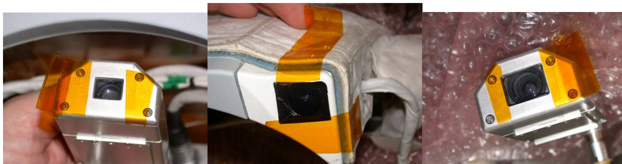
Figure 2 - ERCA lenses covered with Teflon squares and Kapton tape
