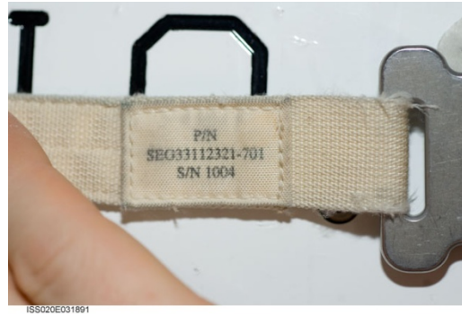
Figure 1c.- Frayed D-ring extender; NO GO for use.
