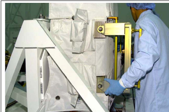
AGB INSTALL ON FHRG – DOUBLE PIN SIDE (MLI FLAPS ARE VELCROED OPEN)
