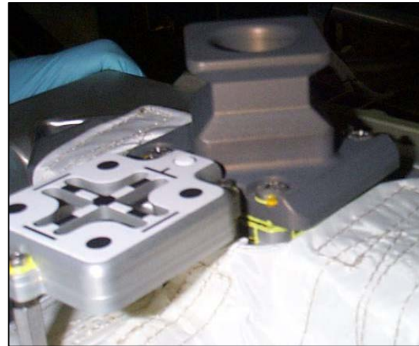
CLPA status indicator (top – indicator shows CLPA not installed, bottom – shows CLPA installed)
