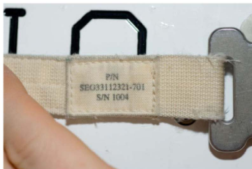
Figure 3. Frayed D-Ring Extender; No-GO for Use.
