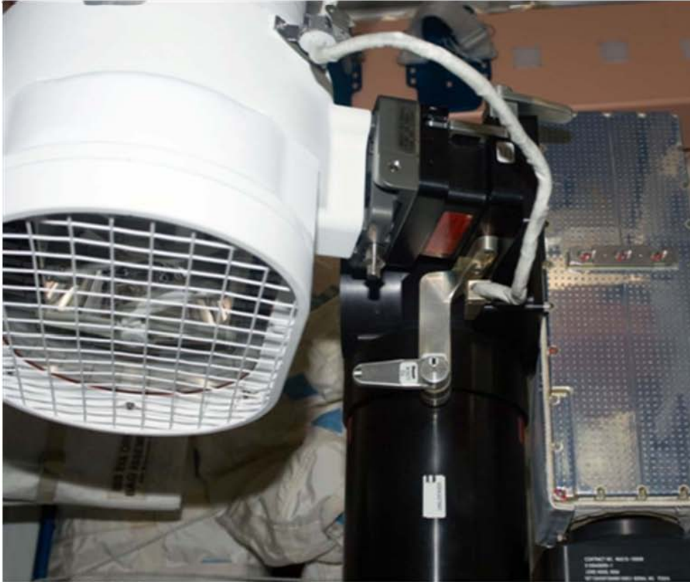
Camera Pan/Tilt Lock (shown in locked position)
