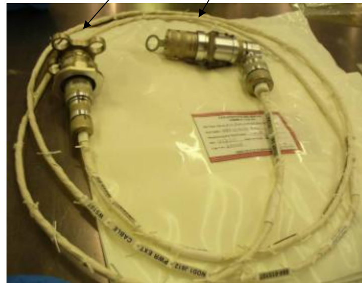
Figure 2.- J612 Extension Cable – Caps Installed.
