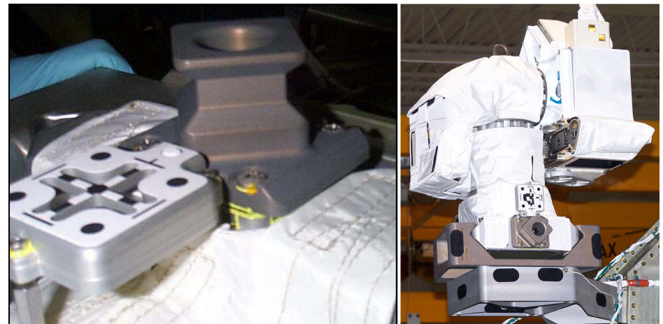
CLPA status indicator (top – indicator shows CLPA not installed, bottom – shows CLPA installed)
