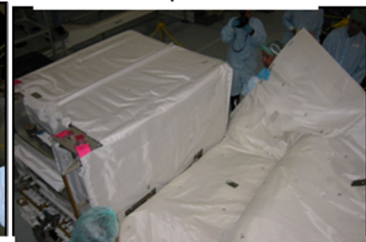
Pull tent away from ESP-2 (stays attached to FSE on port side)
