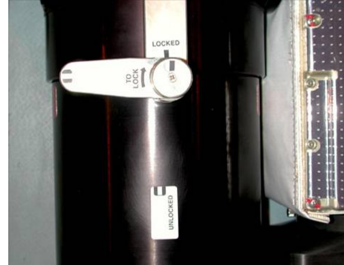
Camera Pan/Tilt Lock (shown in the locked position)
