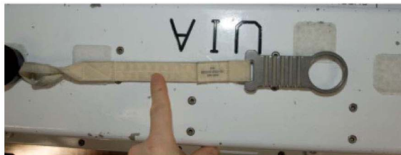
Figure 9. D-Ring Extender Showing Serial Number.
