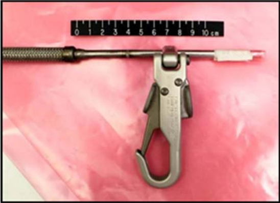
Has equipment hook on 1/4-in nozzle
