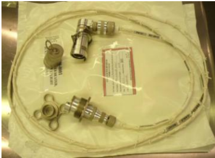
Figure 1.- J612 Extension Cable – Caps Removed.
