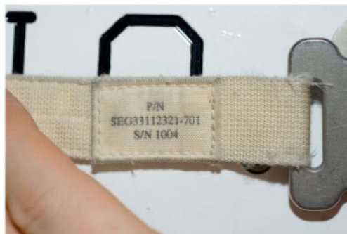
Figure 3. Frayed D-Ring Extender; No-GO for Use.
