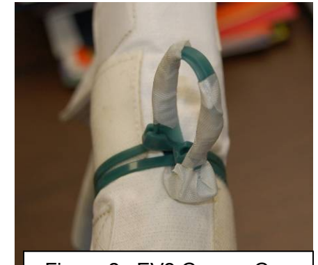
Figure 2: EV2 Grease Gun Wire Tie Config
