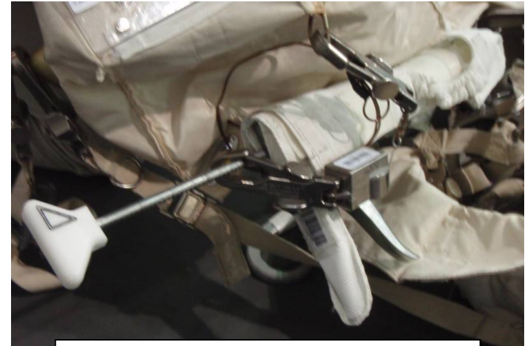
Figure 1: EV1 Grease Gun Wire Tie Config
