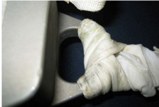
Figure 4. LAS Attachment to ERCM D-Ring.
