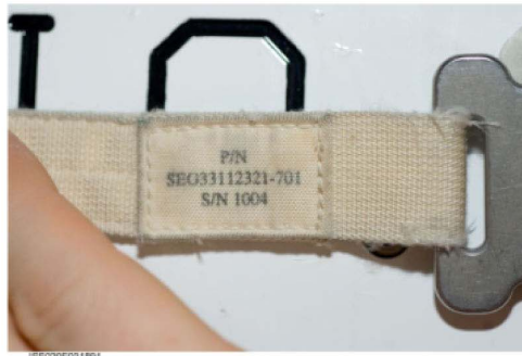
Figure 3. Frayed D-Ring Extender; No-GO for Use.
