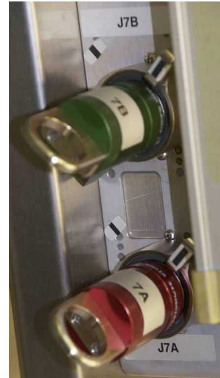
Connectors shown in Lock position
