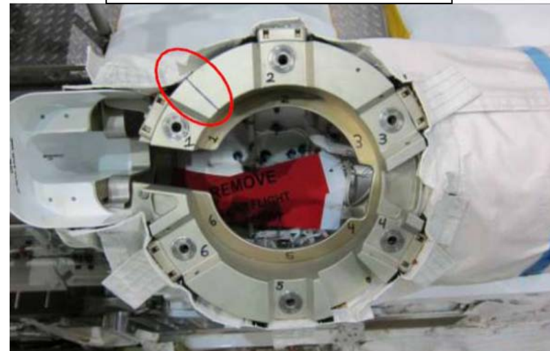
PAA - PDGF Adapter Assembly Black mark at 1 o'clock
