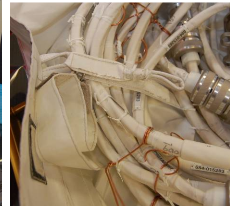
Figure 2: FGB Y-Cable Bag Config Tether through cable, through both D-rings, through bag tether, onto itself
