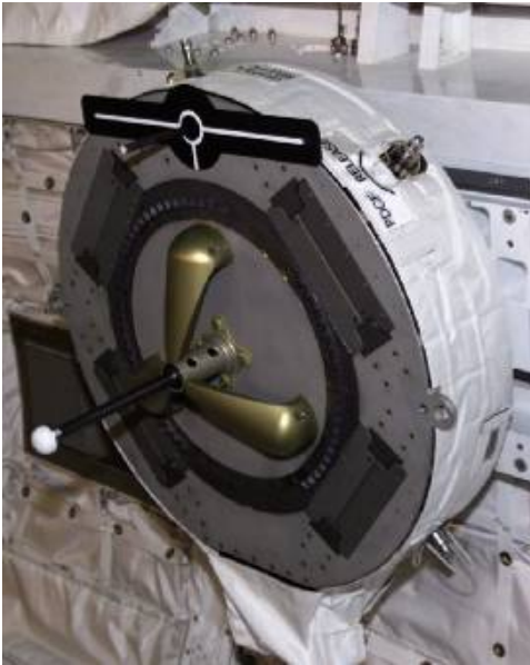
PUMAA – PDGF Universal Microconical Adapter Assembly
