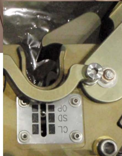
SSBAD – Space Station Boom Attachment Device
