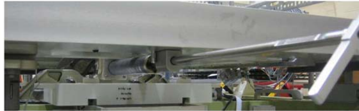
Figure 17. T-Handle Tool Engaged in Removed Capture Bar
