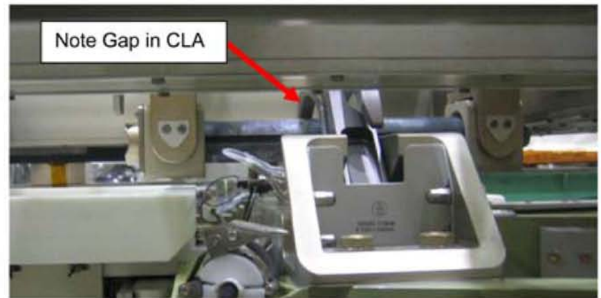
Figure 14.- Capture Bar (Lowered) in Unloaded Position After Driving EVA Interface Knobs.
