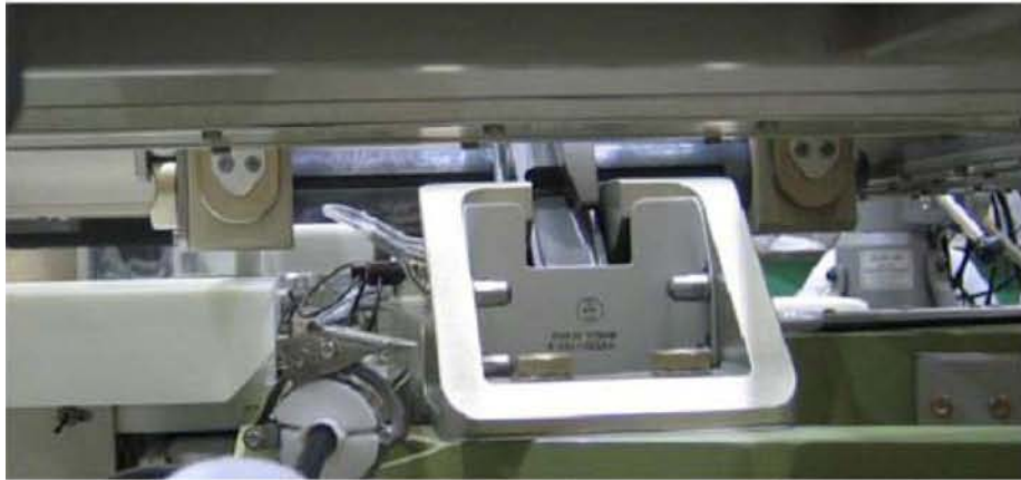
Figure 13.- Capture Bar in Preload Position Before Driving EVA Interface Knobs.
