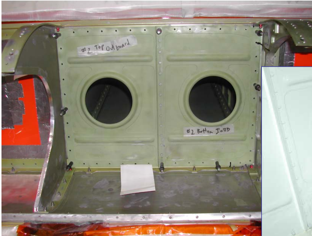
Body Flap Forward Spar After Bead Blasting
