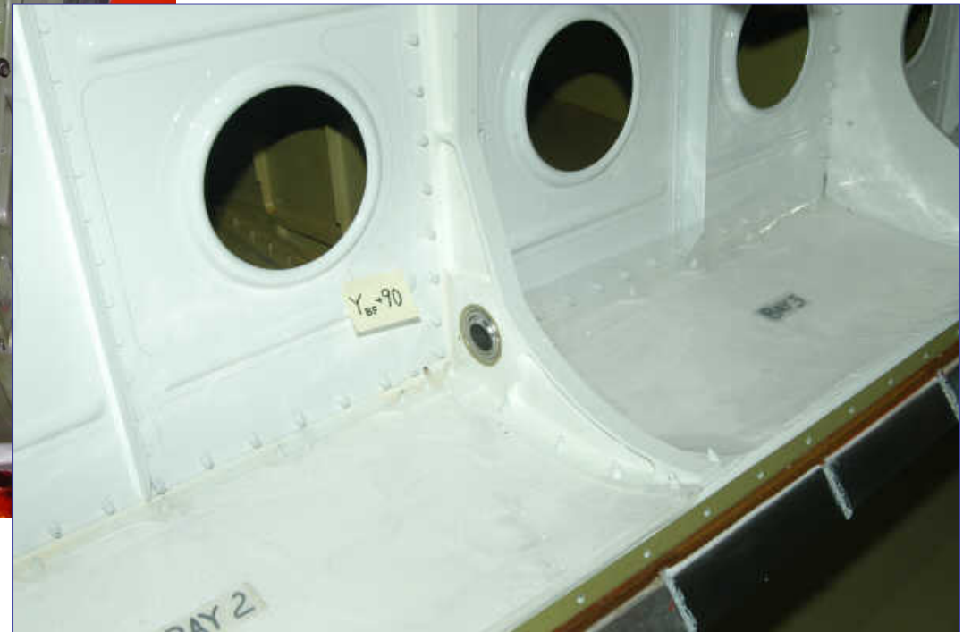
Body Flap Forward Spar After Painting
