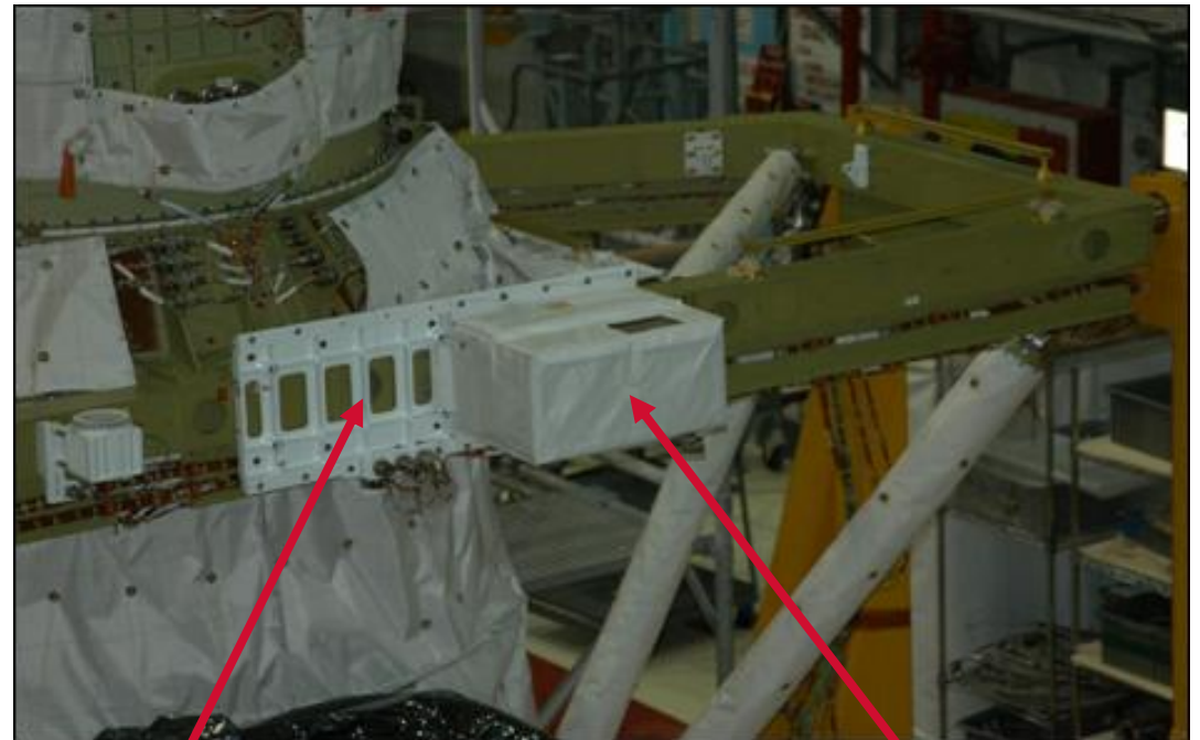
TriDAR Installation Location on Aft Airlock Truss
