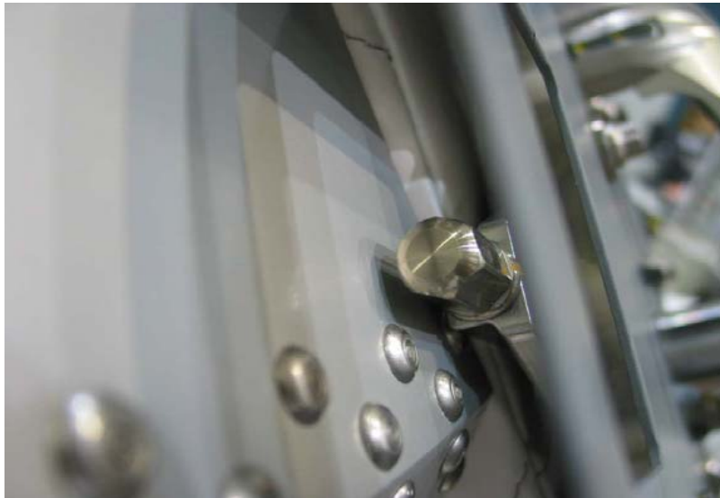
End View of EVA Release Rod/Cupola Interference
