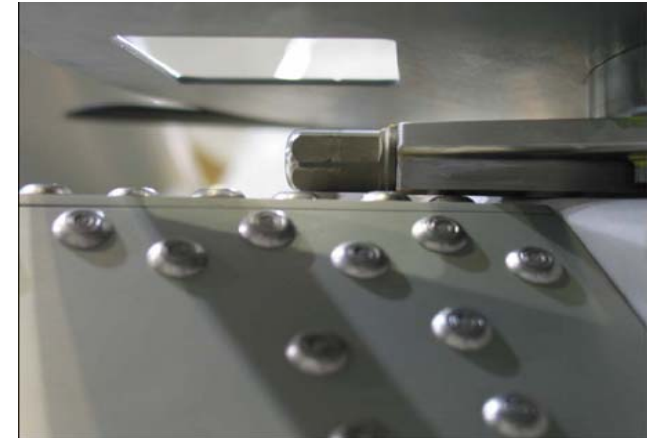
Side View of EVA Release Rod/Cupola Interference
