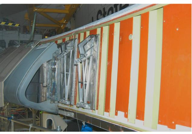
Example of Wing Spar Location (OV104 1-9 spar fitting) During flight 32 processing
