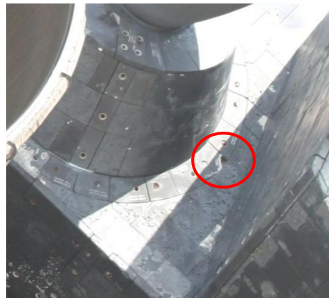
Tile loss from RH OME Base Heat Shield as seen post landing
