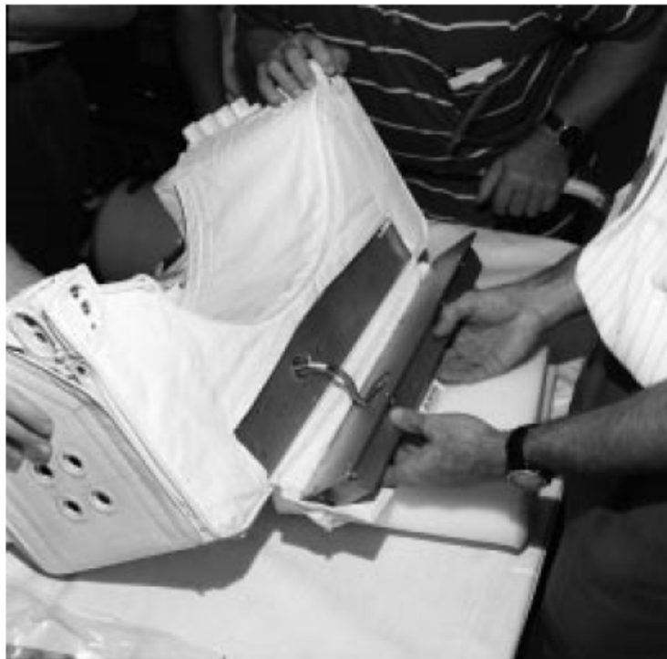
Figure 4.1-16. SAFER battery changeout
