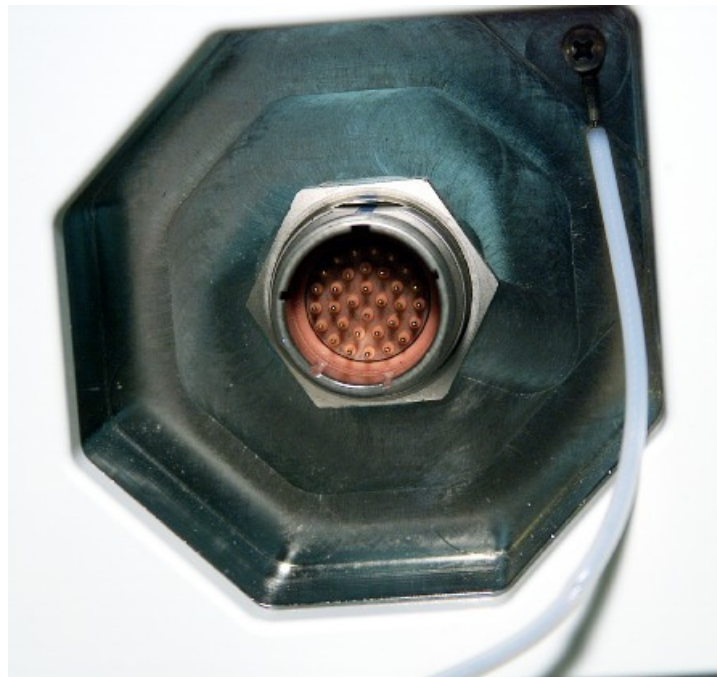
Figure 1.3-8. Auxiliary charge port (uncapped)
