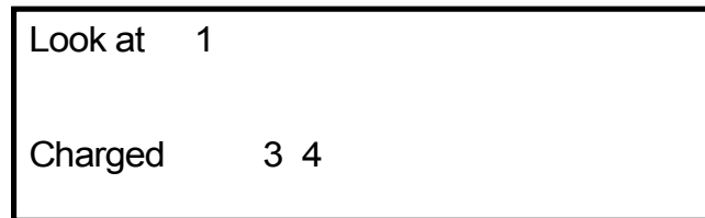
Figure 1.2-8. Battery charger LCD (all channels complete)
