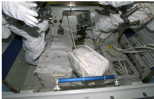
Figure 1.12-2. Equipment lock stowage configuration
