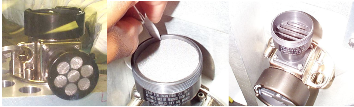
Figure 1.13-21. Removal of the 45 inlet screens on the AMPEV
