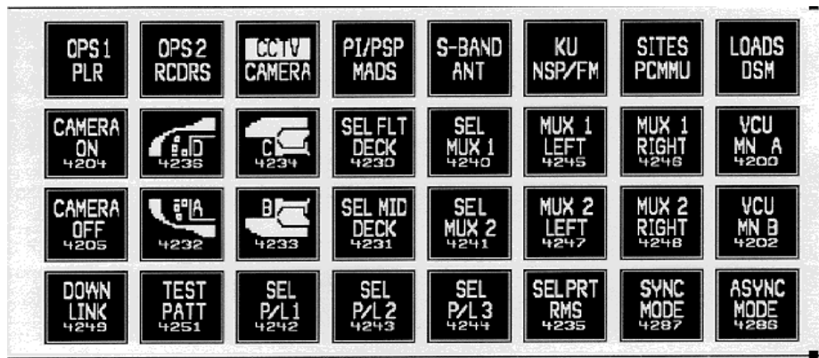
Figure 5.140-4. Example of an MCM panel section
