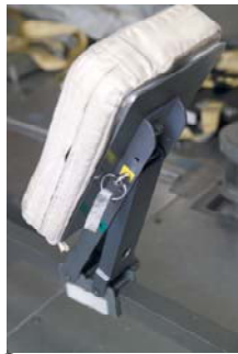
10 Reconfigure seat pip pin and seat assembly from green to yellow. Secure blocks together using Velcro tab. Tighten knob.
