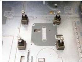
③ Install spacers then sound mounts. Secure loosely with knurled knobs.
