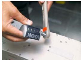
13 Tighten pedals into pedal cranks using wrench if necessary (red = right / blue = left. Note: blue is reverse threaded).
