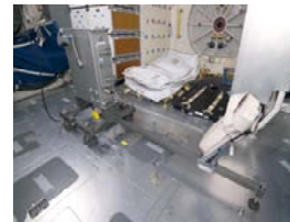
15 Install seat stem foot. Secure with pip pin and tighten by ORB OPS-24b/O/A
