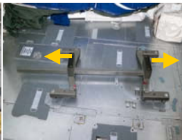
⑥ Release frame from seat 8 deck studs via QDs (4); push button and lift collar. Disassemble frame by sliding seat stem and forward sections apart.
