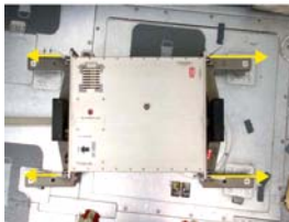
⑤ Remove pip pins (4) securing ergometer to frame and temp stow ergometer.
