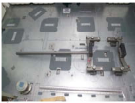
⑧ Loosely secure frame with seat stem onto AQDs with knurled knobs.
