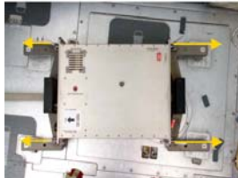
⑤ Remove pip pins (4) securing ergometer to frame and temp stow ergometer
