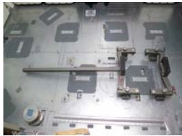
⑧ Loosely secure frame with seat stem onto AQDs with knurled knobs
