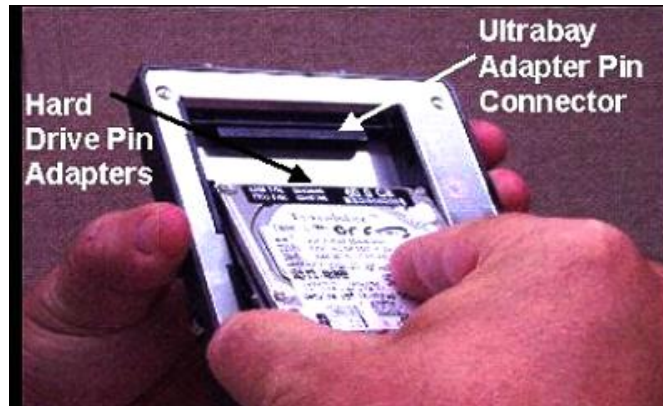
Figure 12-22.- Inserting device into A31p Ultrabay Adapter.
