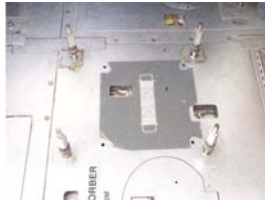
② Secure / latch AQDs onto deck studs
