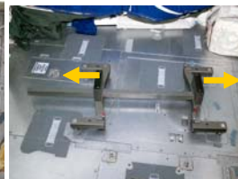
⑥ Release frame from seat 8 deck studs via QDs (4); push button and lift collar. Disassemble frame by sliding seat stem and forward sections apart
