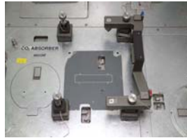
⑦ Loosely secure frame onto AQDs, with knurled knobs
