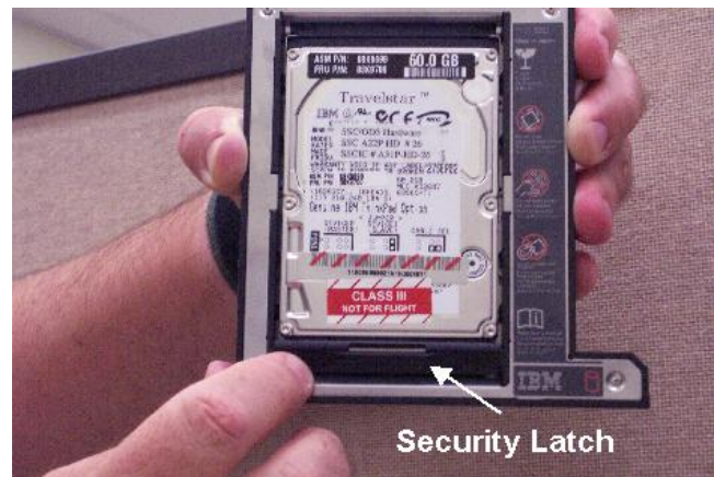
Figure 12-23.- A31p Ultrabay Adapter and A31p Hard Drive final configuration.
