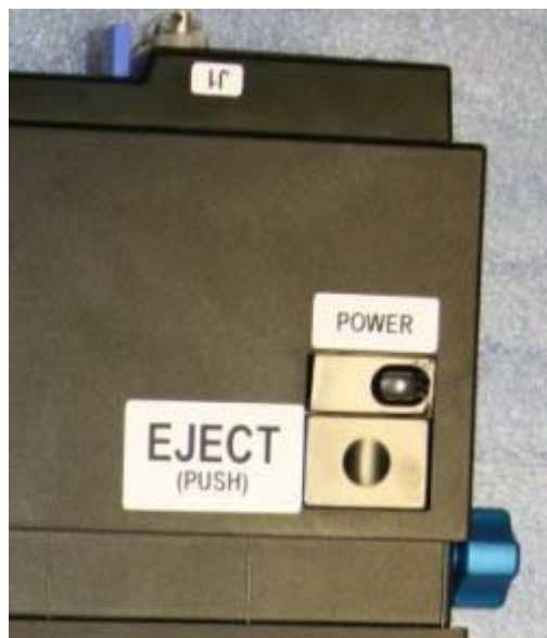
Figure 12-25.- Docking Station Eject button and Power button.
