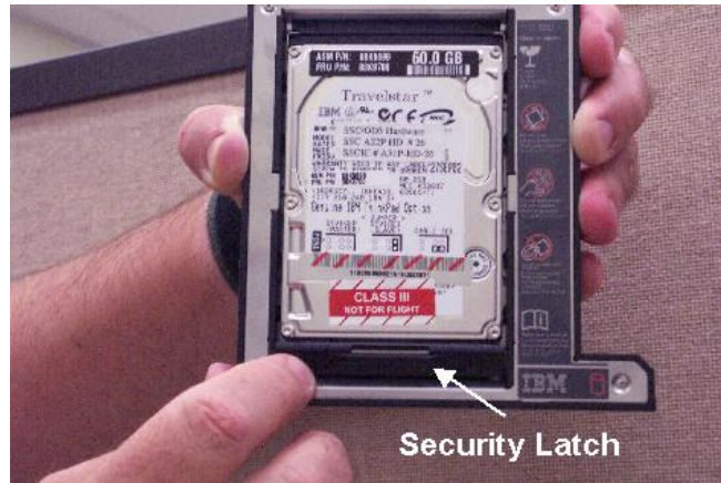
Figure 12-20.- A31p Ultrabay Adapter and A31p Hard Drive final configuration.
