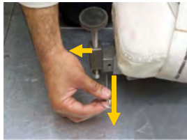
④ Remove pip pin, seat stem foot and seat, temp stow all
