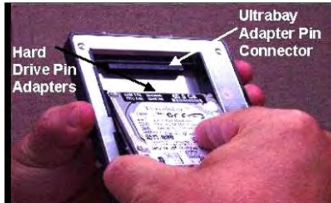
Figure 12-19.- Inserting device into A31p Ultrabay Adapter.
