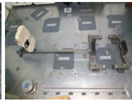
⑨ Install seat onto seat stem
