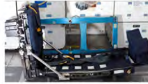
8. Open seat pan into entry config (pull gold T-handles (2) on port and stbd seat back)
