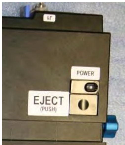
Figure 12-22.- Docking Station Eject button and Power button.
