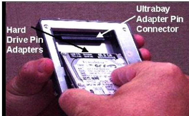
Figure 12-19.- Inserting device into A31p Ultrabay Adapter.
