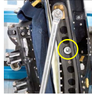
2 Install bushing into port side of seat back. Secure with spring pin
