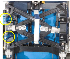
4 Install RSK (blue) ICU brackets (pull spring pin, slide in brackets)
