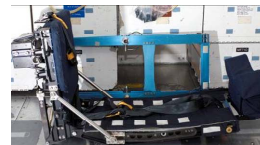
9 Open seat pan(s) into entry config (pull gold T-handles on port & stbd seat back to release seat pan(s))
