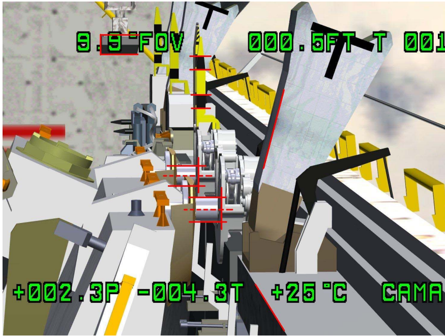
Figure 6-1.- SLP port trunnion view w/ completed overlay (Camera A).
