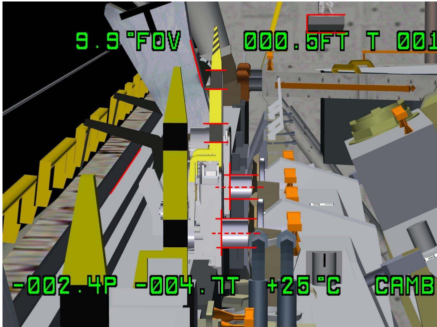
Figure 6-2.- SLP port trunnion view w/ completed overlay (Camera B).
