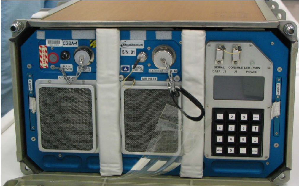
Figure 1: CGBA 4 Locker Insert
