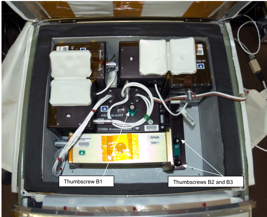
Figure 5: CSI Thumbscrew Locations
