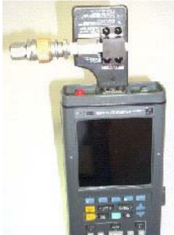
Figure 1.- ISA Scopemeter Pressure Probe Connected to Scopemeter.
