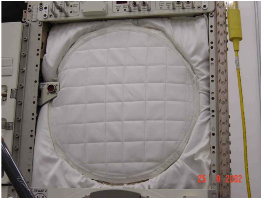
Figure 6.8-2: Acoustic protections in front of BSS after CB Front panel removal
