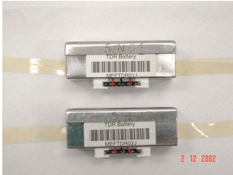
Figure 6.3 - 5: TDR Battery Packs (Only one is stored into the DASE Pouch)
