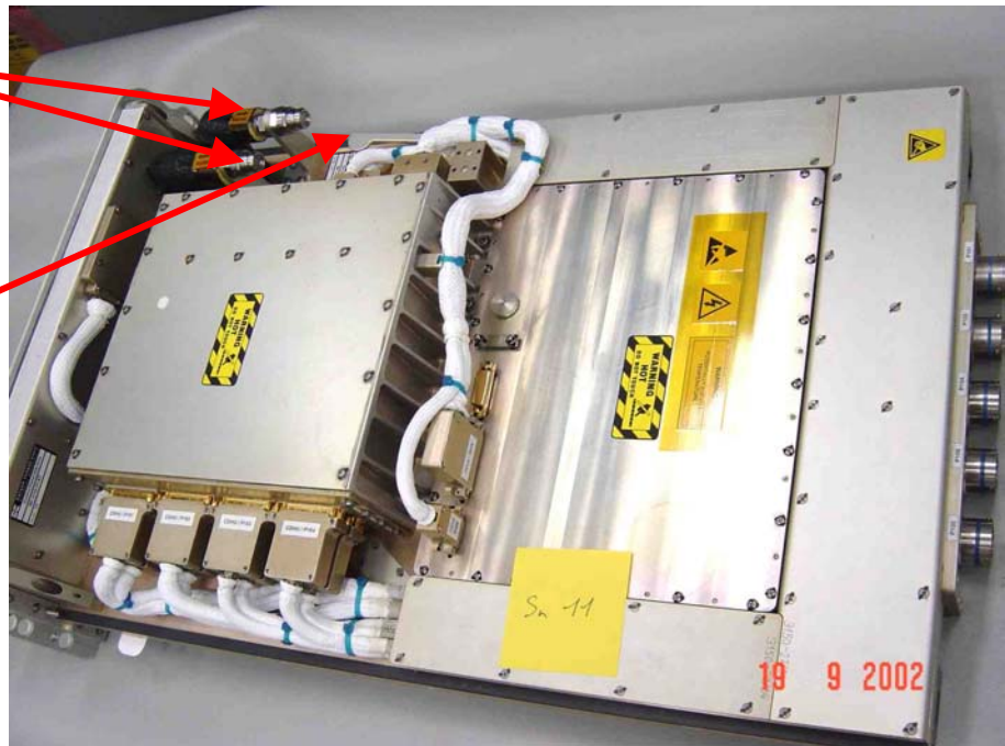
Figure 6.1 - 11: Details of the EU: QDs and end-stop
