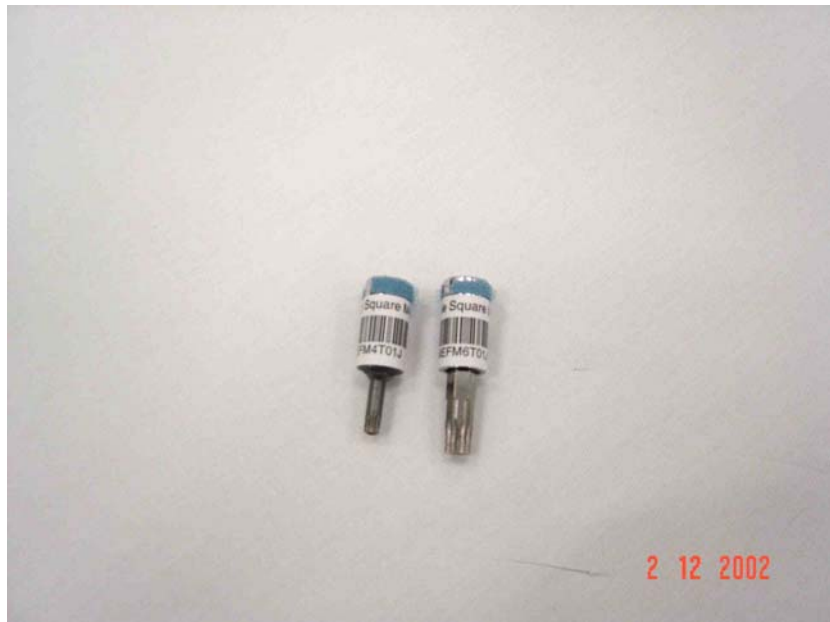
Figure 6.3 - 6: Triple Square M6 and M4 Tools stored into the DASE Pouch
