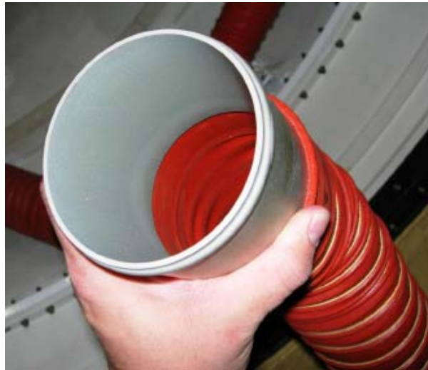
Figure 1-4.- Aft end of Booster Fan Bypass duct for Spacehab (Note: No screen)
