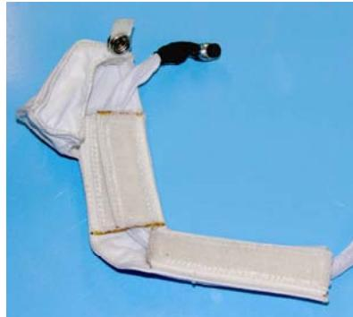
33. Using Velcro, secure Flap 3 to EVA Camr Blanket (DO NOT snap Flap 3)
