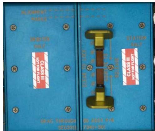
8. Remove Alignment Tool (turn ccw)
