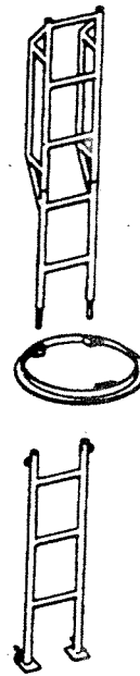
Figure 13-31: LO2 Aft Dome Access Kit (A78-3606)
