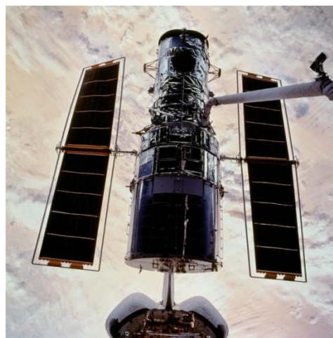
Figure 17.10 HST after RMS grapple, before berthing in Columbia's payload bay (STS-109, March 2002).
