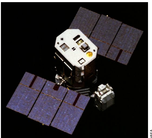
Figure 10.9 Attempted retrieval of the Solar Max satellite by an astronaut flying a Manned Maneuvering Unit on STS-41C (April 1984).
