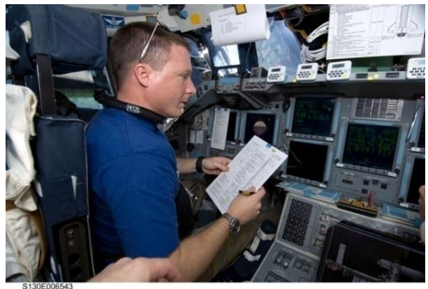
Figure 25.16 Pilot Terry Virts at the commander's station between MC-4 and +R Bar arrival. He is holding the APPROACH cue card. The RNDZ TIGs flight note and the RCS FAILURE/RESPONSE cue card are clamped to the overhead panel in front of him for easy reference. At the lower right of the photo is a laptop running a centerline camera repeater.
