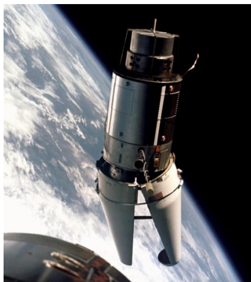
Figure 3.15 ATDA with shroud photographed by the Gemini IX crew (June 1966).
