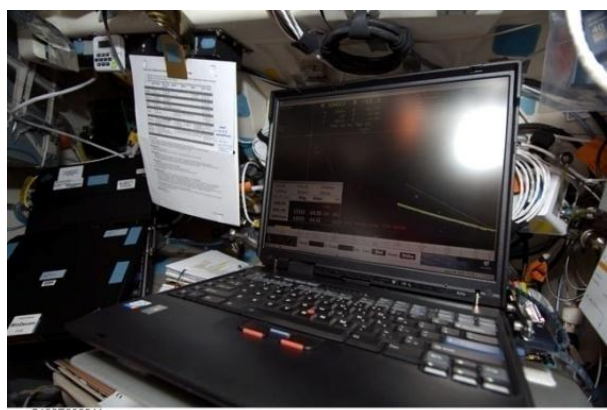
Figure 25.12 RPOP1 (primary) laptop photo soon after the first HHL mark of 15,620.3 feet was taken. Paper to the left of the laptop screen, for easy reference, is a chart (TRAD FAIL RANGE AND RANGE RATE DETERMINATION) that details how the crew should determine range and range rate during proximity operations in the event of sensor failures.
