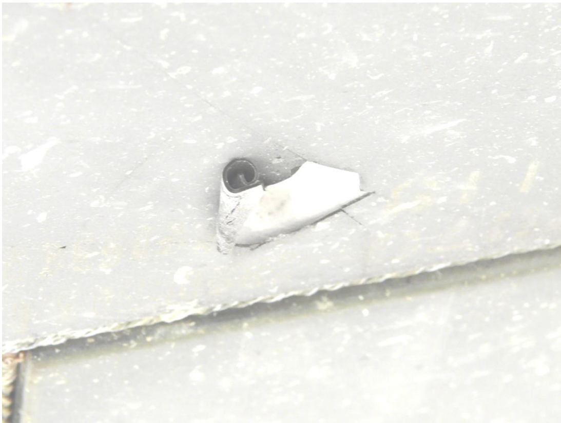
Impact Damage to the Body Flap
